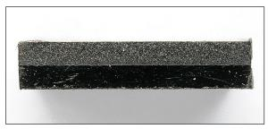
Fig. 1. Cross-section of the explosion welded joint (top layer – Ti, bottom layer – Ni)
